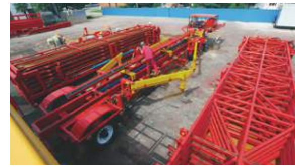
SPC Power Catwalks and Hydraulic Pipe Bin
