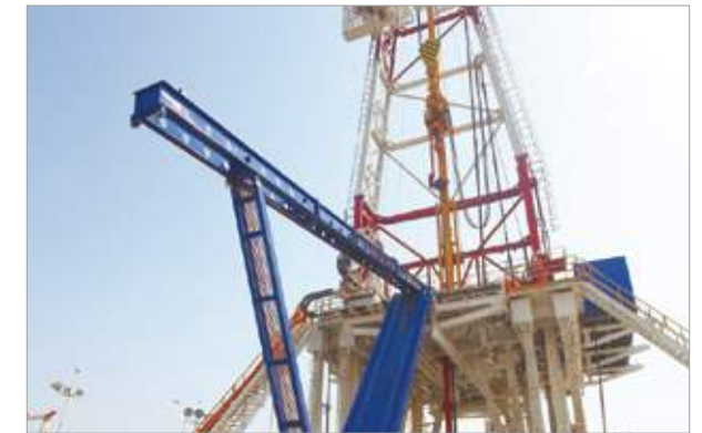
Automated Pipe Feeding System
